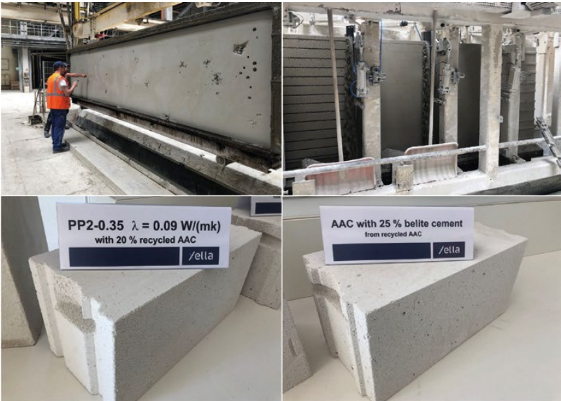
Figure 2: Production of aerated concrete prototypes in the large-scale technical center of Xella Technologie und Forschungsgesellschaft mbH;
