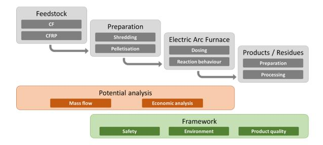
In this project, the principal suitability of the electric arc furnace (ELBO) for recycling carbon fibers (CF) and carbon fiber-reinforced plastics at the end of their life cycle will be examined.
