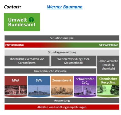
As part of the project, various thermal processes were investigated with regard to their suitability for the energy or feedstock recycling of waste containing carbon fibers. The focus of the measurements at the large-scale plants was on determining the potential fiber load of the process-specific residues and products.
